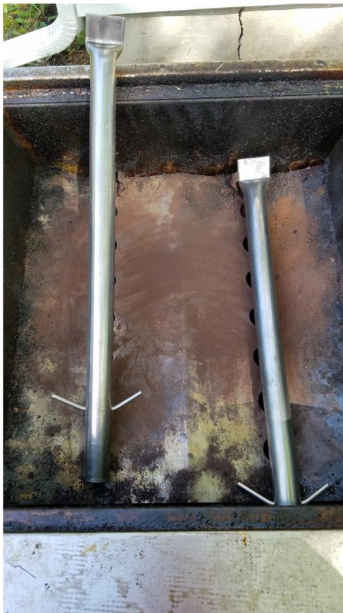
6. Insert tube into hole in front of wall carefully pushing down on back of tube.
