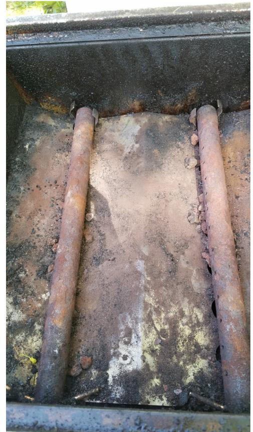
3. Pick up the burner just in front of the opened bracket and gently lift at an angle - carefully sliding the front portion out of the hole in the front wall
